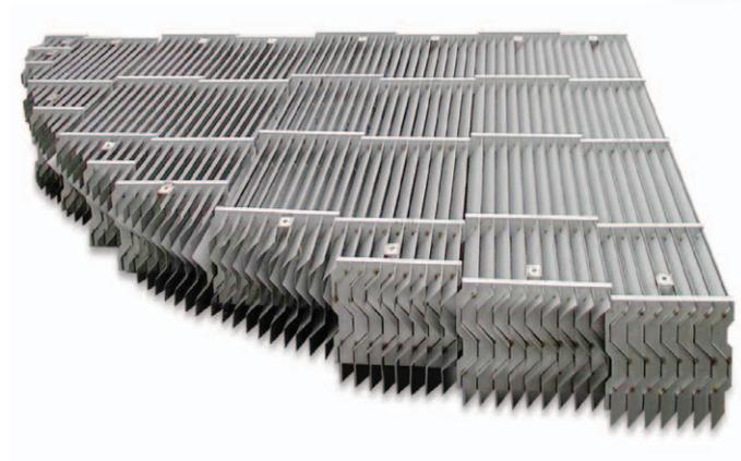
Complex Vane Pack designs provide special separation channels to allow disengagement of liquid and drainage from the vane surface which increases the capacity. These profiles are therefore used when equipment size is critical, for example in de-bottlenecking of existing equipment.
