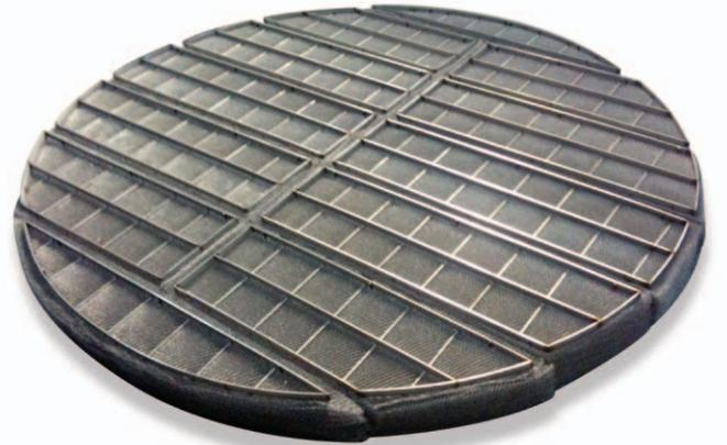
They are produced as multiple layers of knitted mesh making it a dense pack and presenting a large surface area to the droplets entrained in the gas stream. The separation of the droplets is achieved by impingement on, and capture by, the wires of the mesh where the droplets coalesce and drain.
